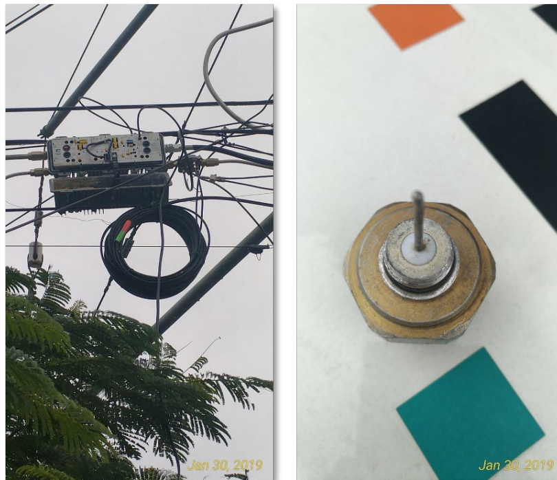
Figure 32. Amplifier [2] with corroded connector (courtesy of Akleza).
