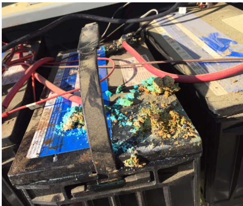
Figure 15 – Battery Corrosion
