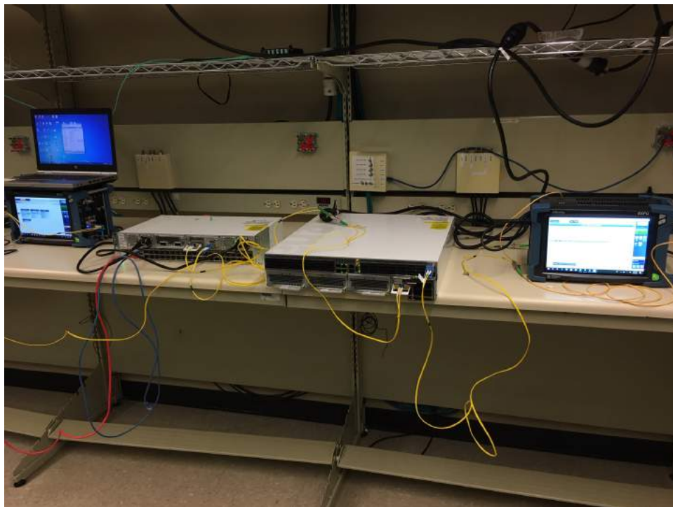
Figure 14 – EXFO traffic generators with Ciena switches
