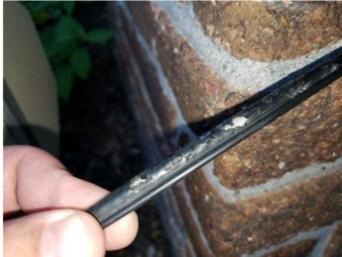
Figure 22. Damaged coax jacket where water was able to enter the cable.
