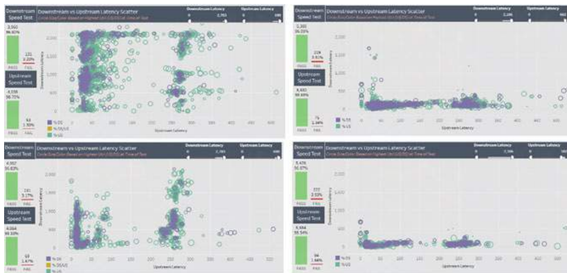
Figure 44 - Maximum, Minimum and Mean DS and US LUL with (Left) High Target Latency Values for DS AQM and (Right) Optimized Target Latency Values for DS AQM
