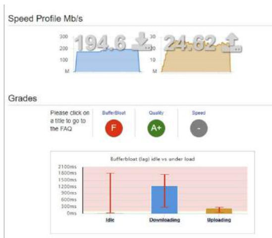
Figure 6 – Left: dsreports.com results with suboptimal DS AQM settings and D3.1 CM with BC with 250ms default target latency; Right: Optimized DS AQM settings and D3.1 CM with US AQM with 10ms default target latency
