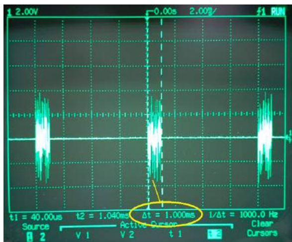
Figure 20 - CW test burst in time domain and spectrum of CW bursts
