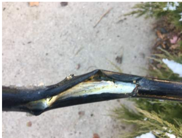
Figure 43. Damaged hardline coax that was at one end of an echo tunnel; the other end was a loose seizure screw on a chassis terminator installed in an end-of-line tap. Further
