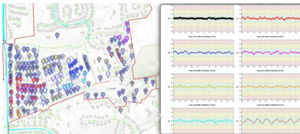
Figure 40 - Upstream Adaptive Pre-Equalization Analysis; Echo Response Groups, Mapped
