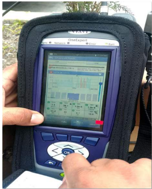
Figure 31. Fault still visible after replacement of amplifier [1] (courtesy of Akleza).
