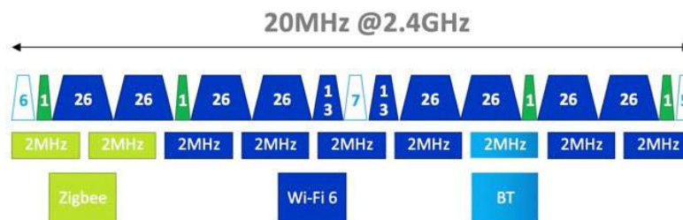
Figure 40 - Improved Wi-Fi 6 IoT co-existence with ZB/BT
