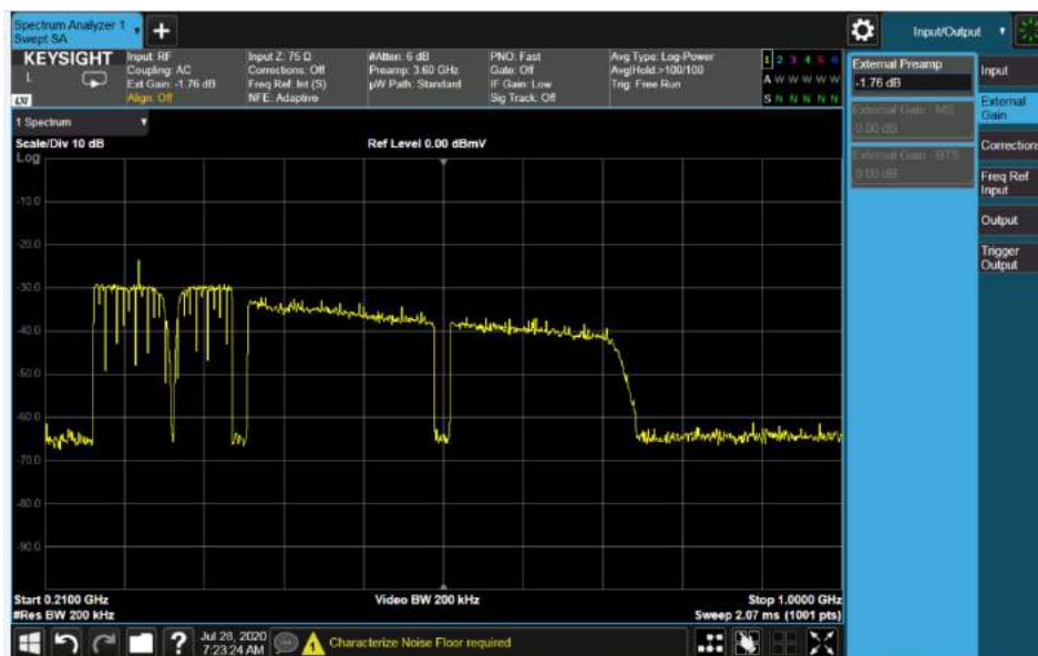
Figure 5. Spectrum analyzer display of the same RF spectrum in Figure 4 (courtesy of CableLabs).
