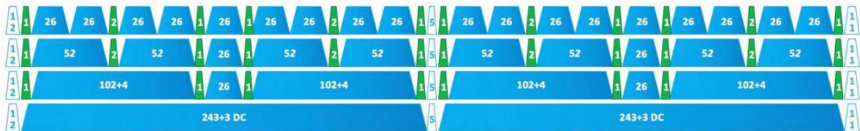
Figure 12 - 40MHz RU allocation mapping
