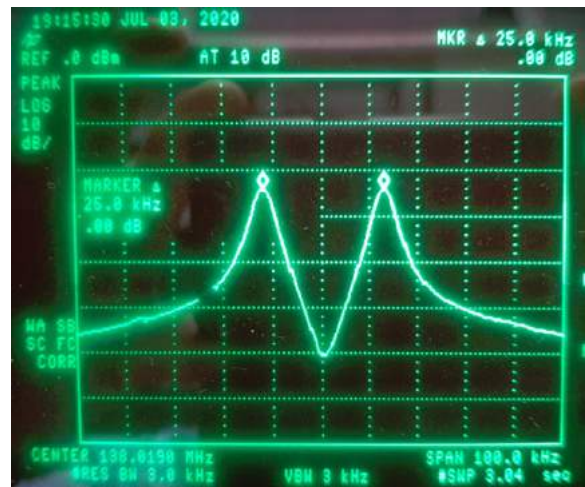
Figure 20 - CW test burst in time domain and spectrum of CW bursts
