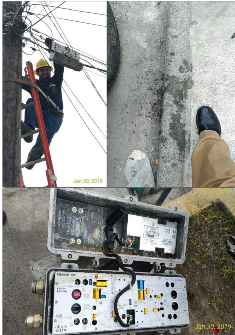
Figure 30. Amplifier [1] containing water and showing corrosion (courtesy of Akleza).
