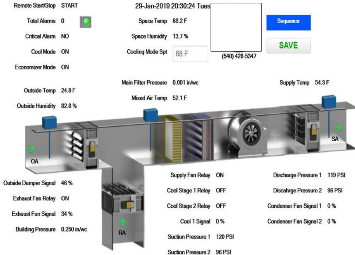
Figure 14 - Aaon Dashboard With Operational Performance Of Economizer
