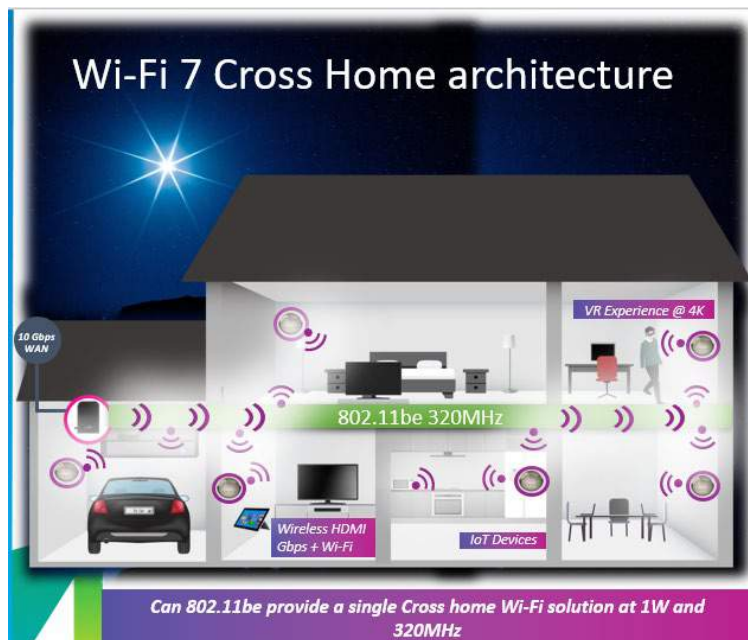
Figure 29 - Basic single 30dBm - 8x8 or 4x4 Cross Home Wi-Fi 7 Architecture
