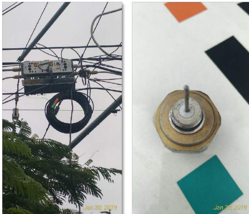
Figure 32. Amplifier [2] with corroded connector (courtesy of Akleza).
