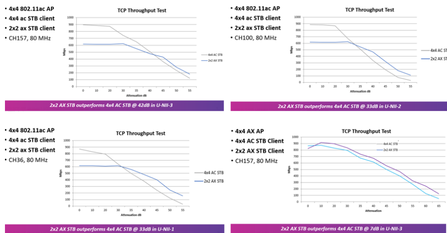
Figure 16 - STB client performance showing 2x2 Wi-Fi 6 outperforming AC 4x4
