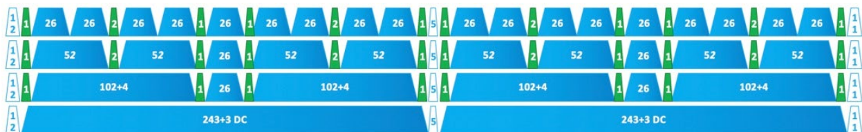
Figure 12 - 40MHz RU allocation mapping
