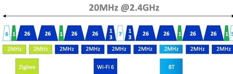
Figure 40 - Improved Wi-Fi 6 IoT co-existence with ZB/BT
