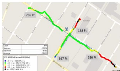
Figure 12 Field Drive Test Plot
