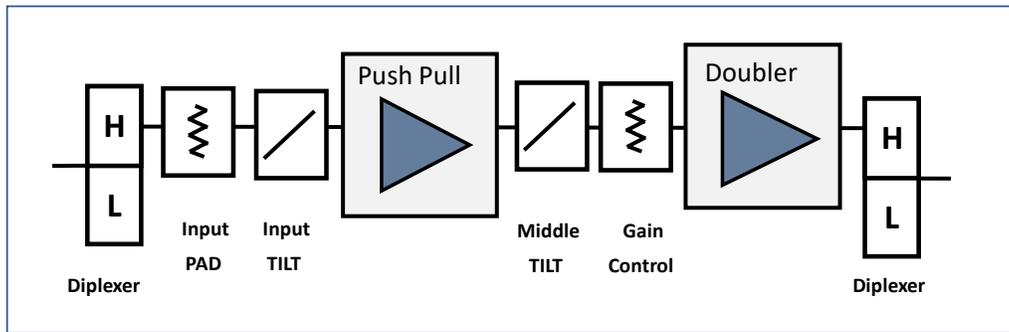
**Figure 1 – Simplified Downstream Line Extender**
