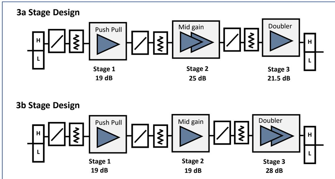
**Figure 5 – High Gain 3-Stage Design Options**
