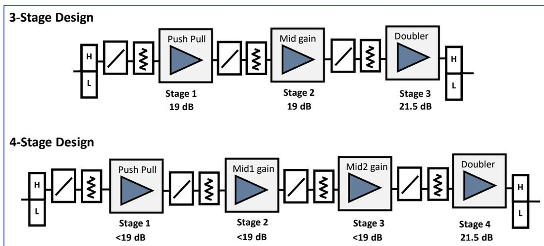
**Figure 4 – Options for Increasing Downstream ES Gain**
