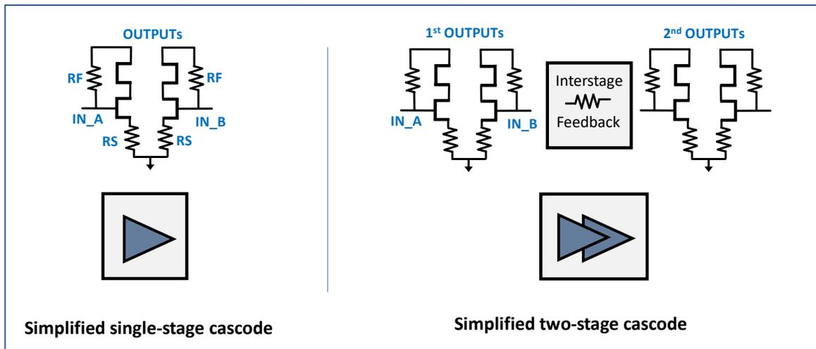
**Figure 2 – Single and Two-Stage Cascode Amplifier Component Topologies**
