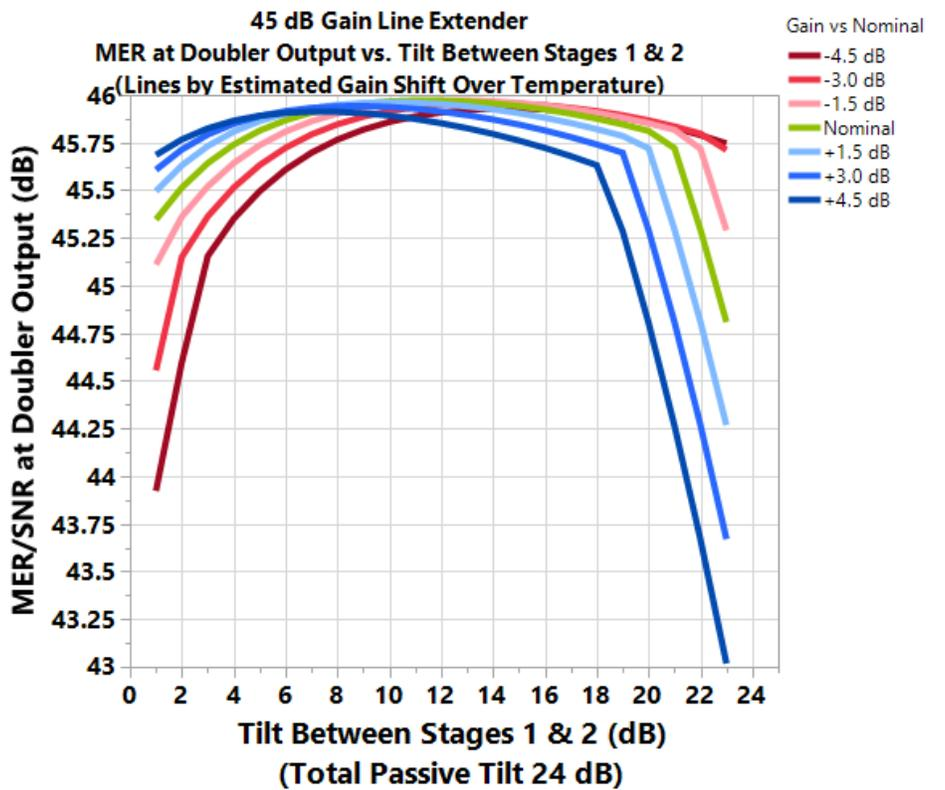
Figure 11 – Modeled MER Performance of 45 dB Line Extender
