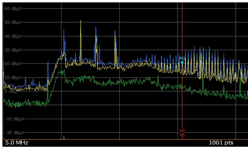
**Figure 1 A Snapshot of Upstream Interferences in an HFC Network**
