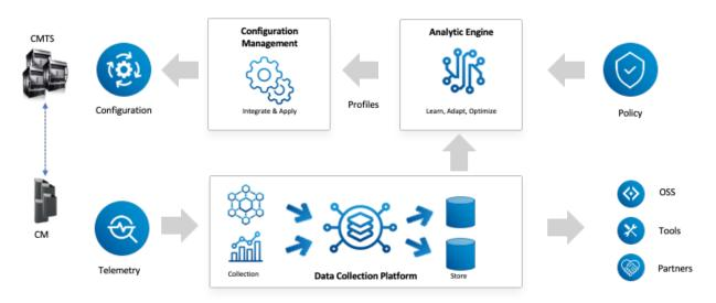
The first step of the Octave process is data collection, done by the data collection platform, which is internally named Genome. The purpose of this service is to poll both CMTS and cable modem telemetry data, sanitize it, aggregate it, and store it in a data lake for further use. In the case of Octave, the consumer of this data is the Analytic Engine (AE). For the purpose of this publication, this service will be treated as a black box, but interested readers can delve into the details in *A*
