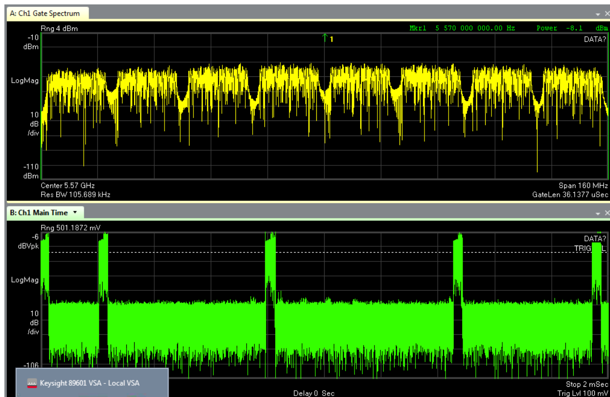
Figure 14 - 802.11a signal are still used in Wi-Fi 6, here for Block ACK
