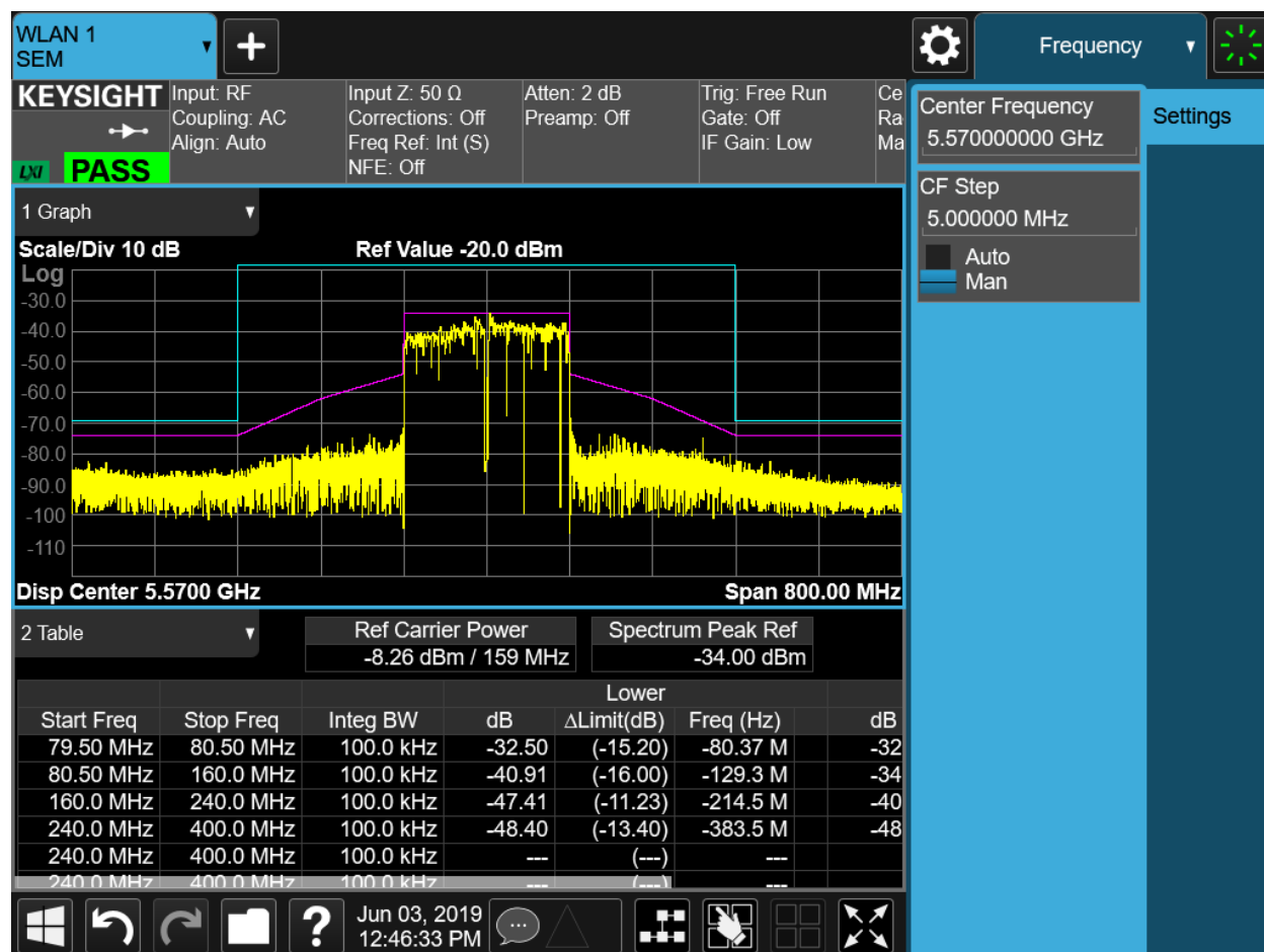
Figure 7 – Primary channel 100 with channel width 160 MHz center frequency 5570 MHz
