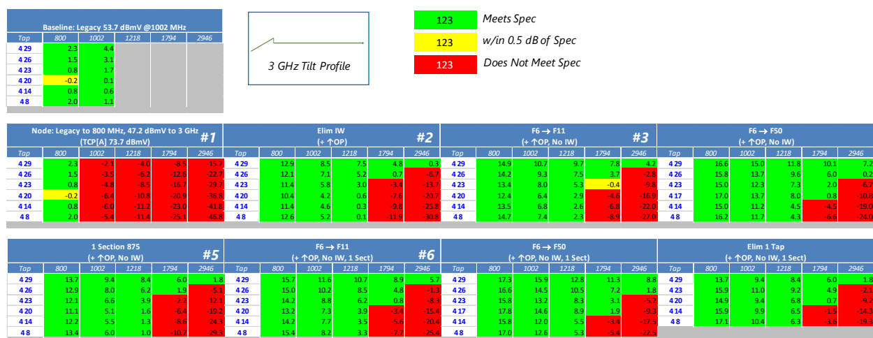
Figure 11 - End-of-Line Signal Levels for 3 GHz Plant Extension (800 MHz Step-Down)
