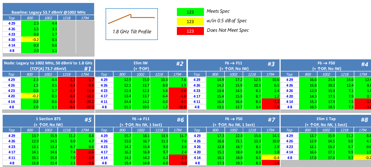
Figure 9 - End-of-Line Signal Levels for 1.8 GHz Plant Extension (1002 MHz Step-Down)
