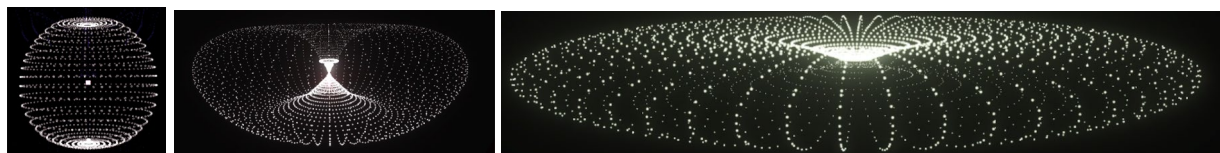
Figure 15 A, B, C RF radiation patterns for Isotropic radiator, low gain dipole and high gain dipole
