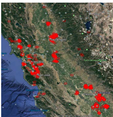
Figure 23 LoRaWAN coverage map on HFC with gateways and antennas mounted ~21 feet high
