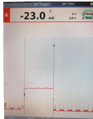
Figure 8 A and B LoRaWAN mote #3 transmit demand on the 6VDC battery from both a power and time perspective
