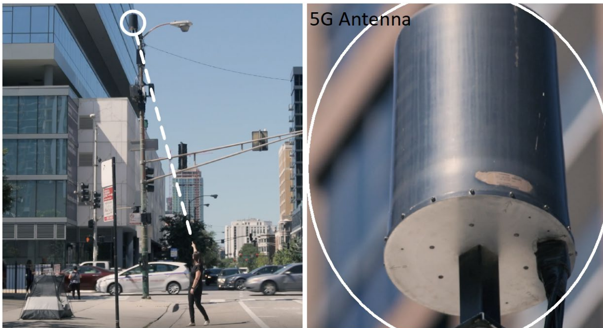
Figure 10 Radio Access Network showing 5G Cell Site with mmWave
