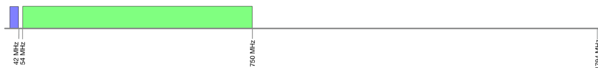
Figure 1 – North American spectrum usage; 42 MHz return split and forward to 750 MHz
