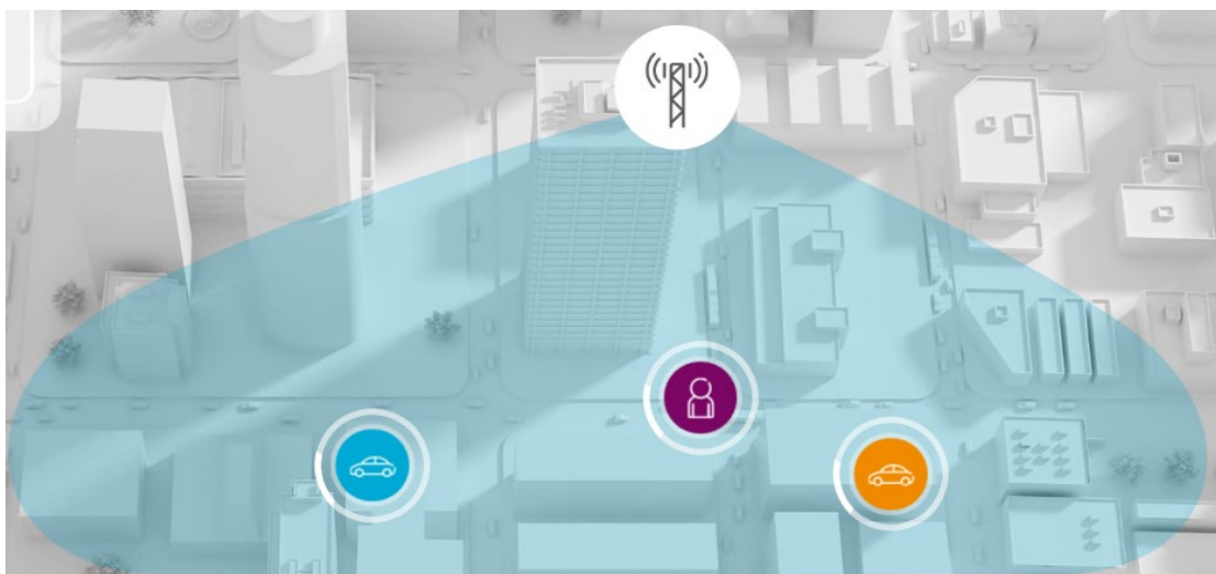
Figure 4 - Coverage under broadcast beam
