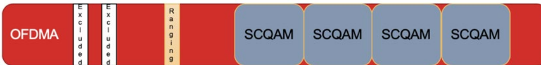
Figure 36 – OFDMA Channel configuration example
