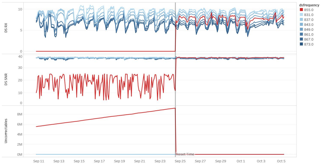
Figure 2 - The ROCK Fixing a Modem With a Single Channel Impairment
