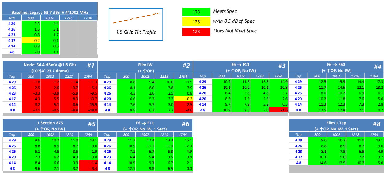
Figure 10 - End-of-Line Signal Levels for 1.8 GHz Plant Extension (Linear)
