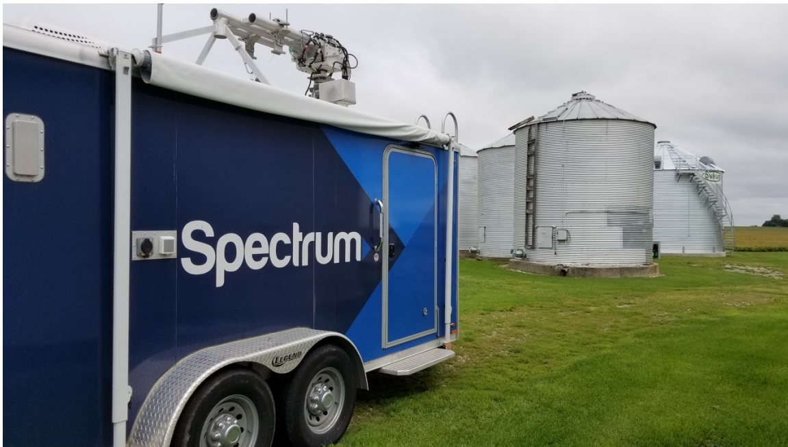
Figure 5 - Wireless field test trailer with extendable radio mast for 5G NR and EPC equipment
