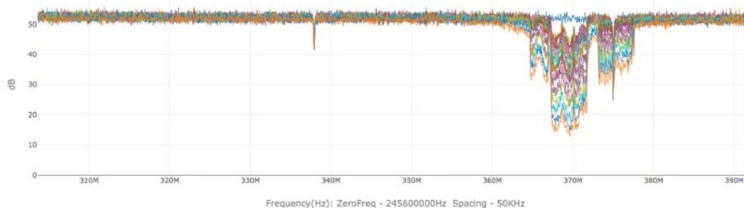
Figure 16 – D3.1 DS RxMER plots w Noise Injection LTE signal (3 channels)
