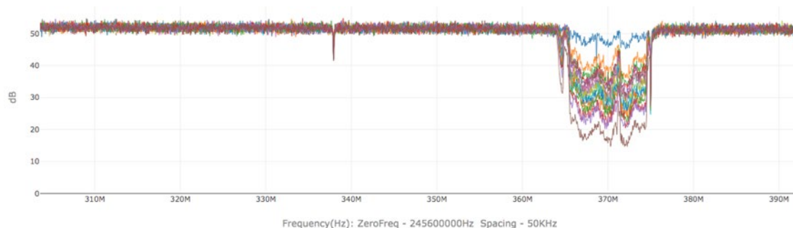
Figure 14 –D3.1 DS RxMER plots w Noise Injection LTE signal (1 channel)
