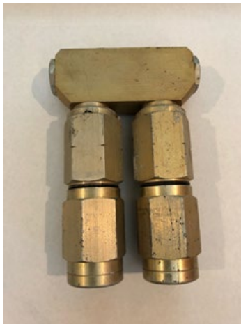
Figure 29. Trunk splice removed from network.
