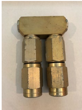
Figure 29. Trunk splice removed from network.
