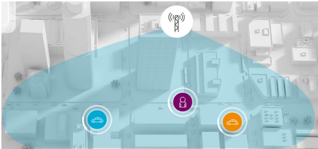
Figure 4 - Coverage under broadcast beam
