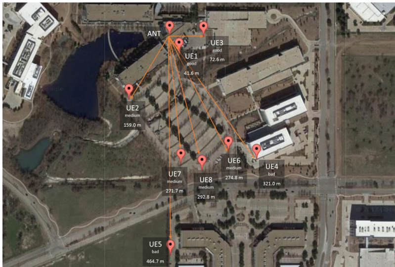
Figure 10 - Setting for MU-MIMO field testing in varying radio conditions
