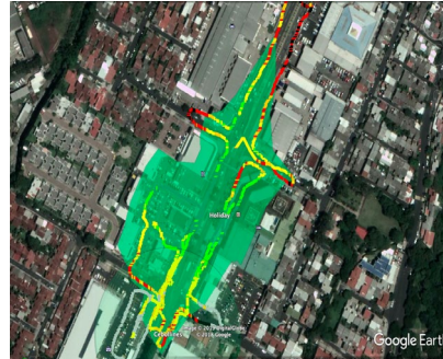
Cell Diameter: 312m Cell Radius: 156m Cell Area (m): 22,304m 2 Cell Area (ft): 240,076 sq.-ft
