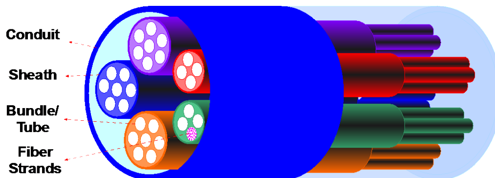
Figure 2 – Schematic Representation of Fiber Sheaths in Conduit
