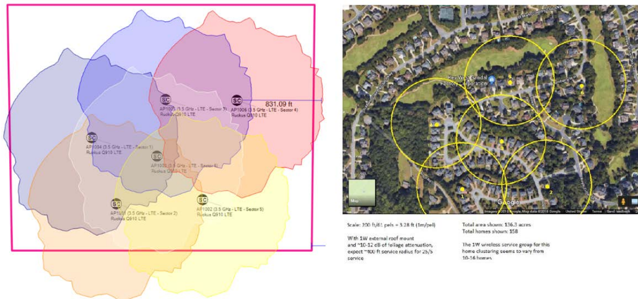
Figure 27 - 1 W HaaT Simulation Vs Calculation; ~ 2:1 Service Radius Improvement in Sim
