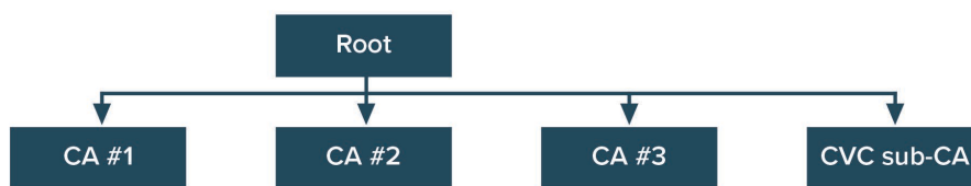
Figure 10 - Using Managed PKI to Create Separate Sub-CA Branch to Sign Code
