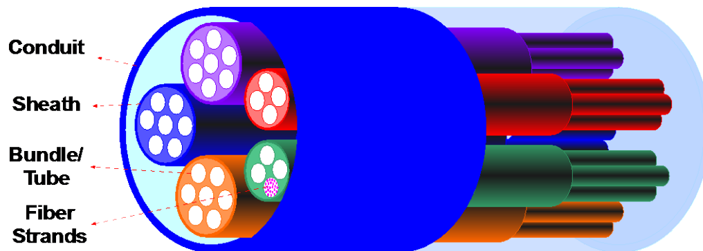
Figure 2 – Schematic Representation of Fiber Sheaths in Conduit
