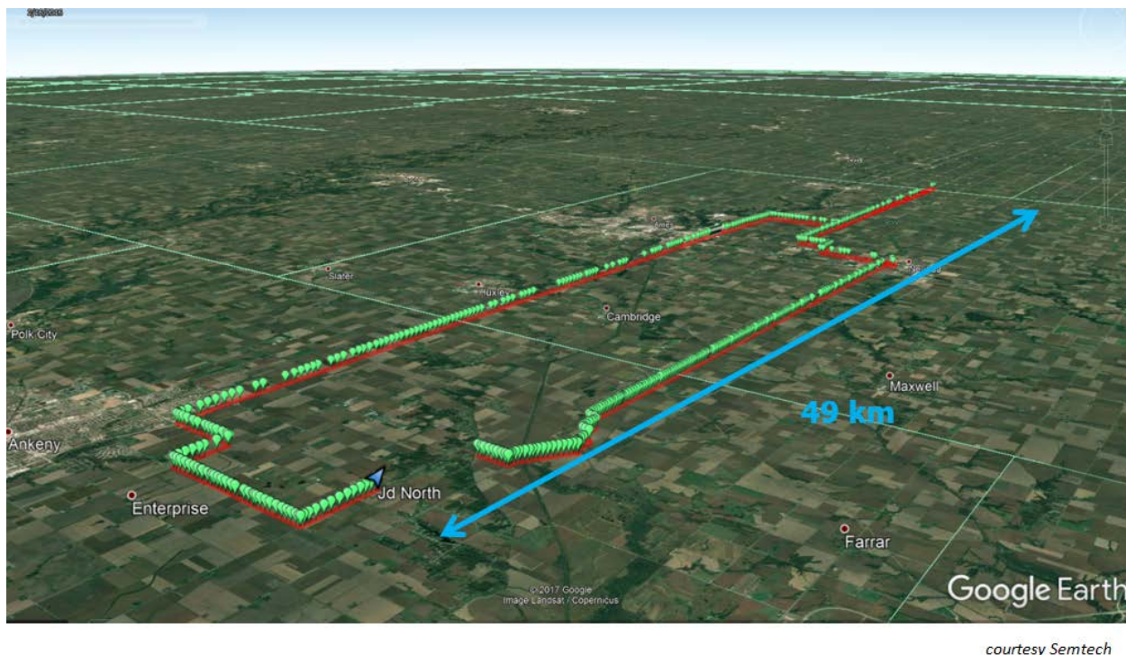
Figure 38 - Sample LoRa Rural Mobile Inside/Out Lossless Connectivity @ 49 Km (!) Radius
