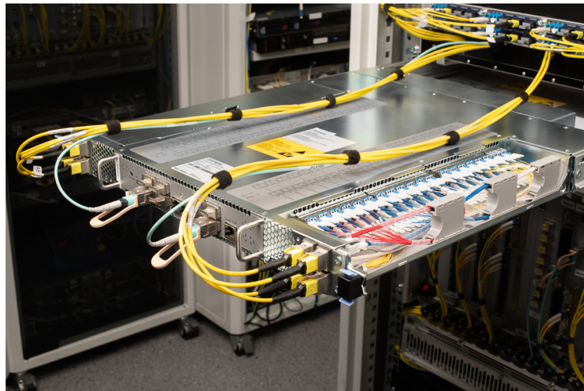
Figure 3 – Packet-Optical System With MPO-Based 10G Connectivity
