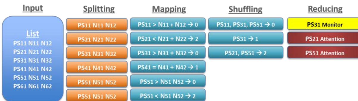
Figure 11 - MapReduce Functions for Heat Map Application
