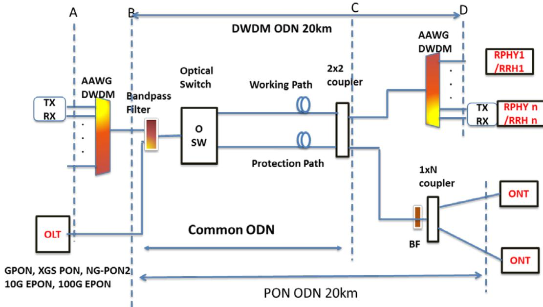
**Figure 6 - A novel DWDM with PON overlay architecture**
