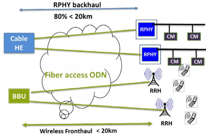
**Figure 5 - Fiber networks for RPHY backhaul and 5G wireless fronthaul**
