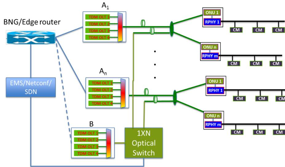
Figure 9 - PON for RPHY Backhaul with Protections
