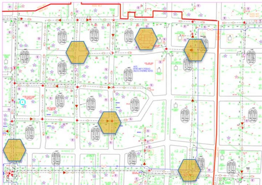
**Figure 8 – 500 foot small cells integrated with HFC network**
