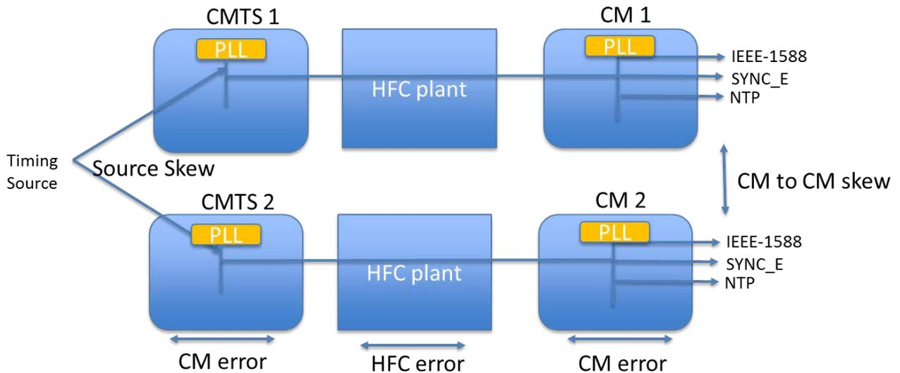
**Figure 5 - DTP System Skew And Error Budgets**
