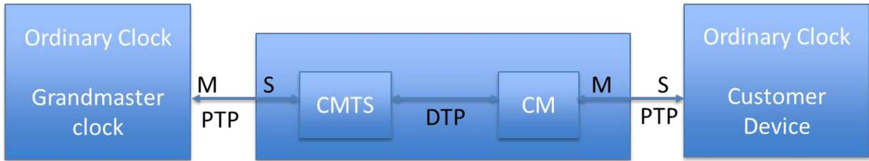
**Figure 4 - DOCSIS System Works Like Boundary Clock**
