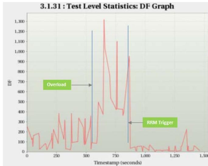
**Figure 9 - Band Steering – Impact on Delay Factor**
