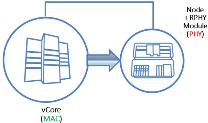
**Figure 7 - Remote PHY with Virtual Core**
