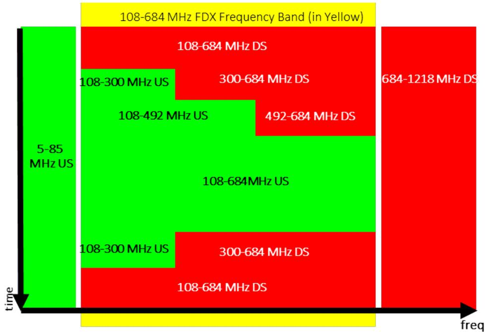
**Figure 10 - Dynamic FDD Operation from cable modem perspective**
