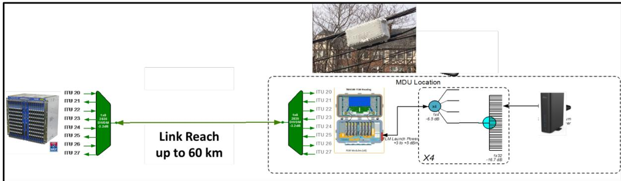
**Figure 7 – 10G / 10G EPON Extender Network Configuration**
