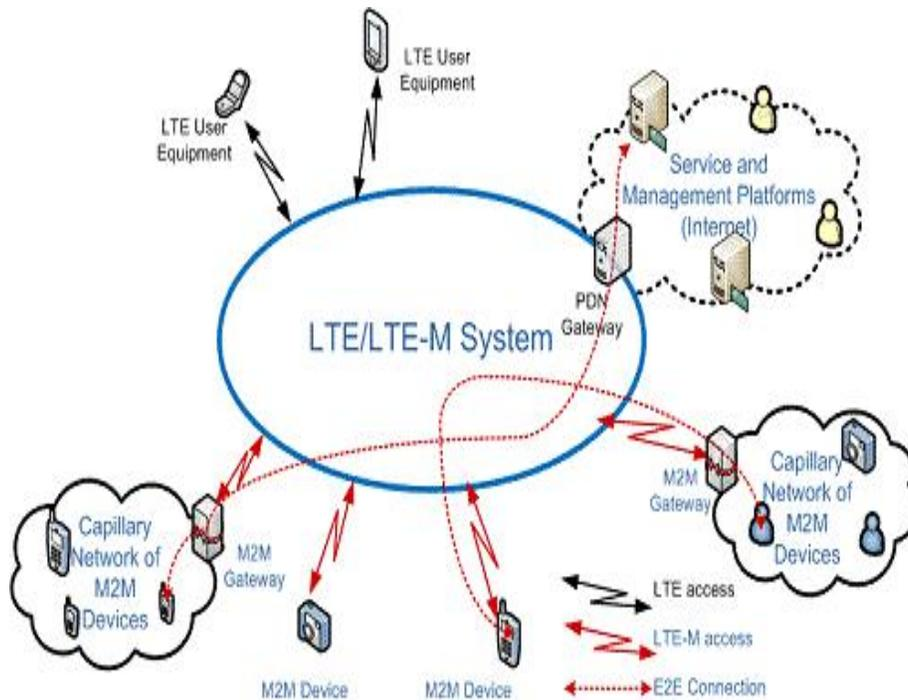
**Figure 12 - LTE-M System diagram**
