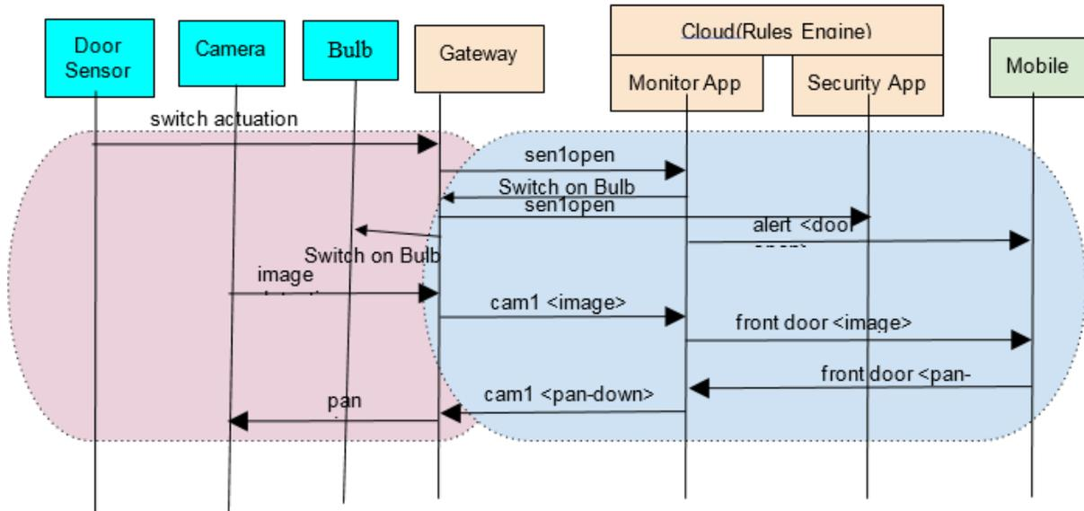
**Figure 8 - Sample Sequence Diagram of IoT Use Case**
