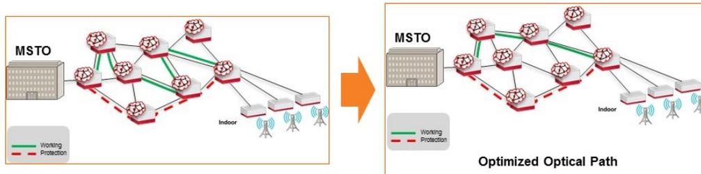
**Figure 11 - Optimized Optical Path**
