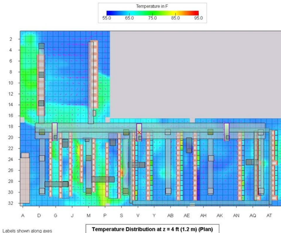
**Figure 7 - CFD Model Results After Airflow Optimization**
