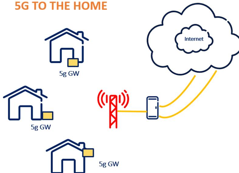
**Figure 2 – Fixed Wireless Access using 5G**
