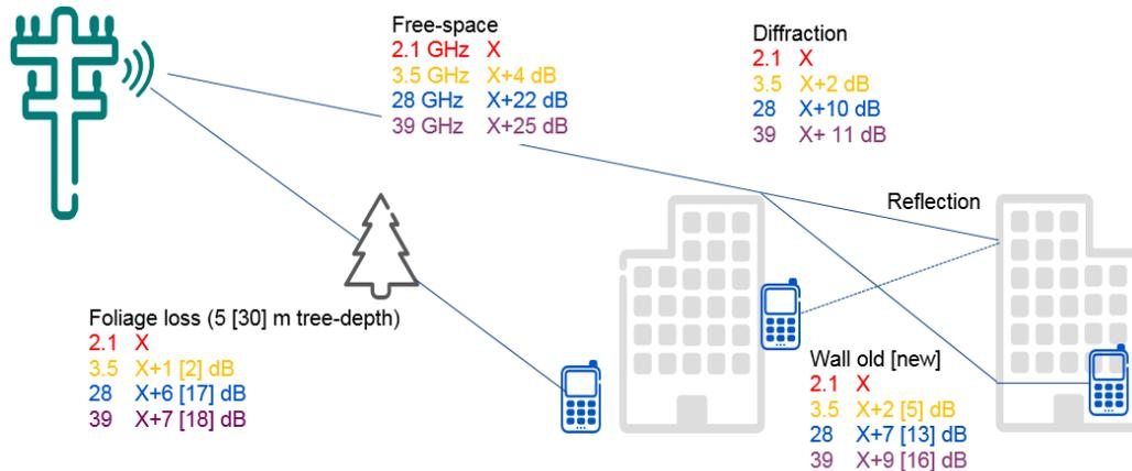
**Figure 4 – Path loss comparison between spectrum bands**
