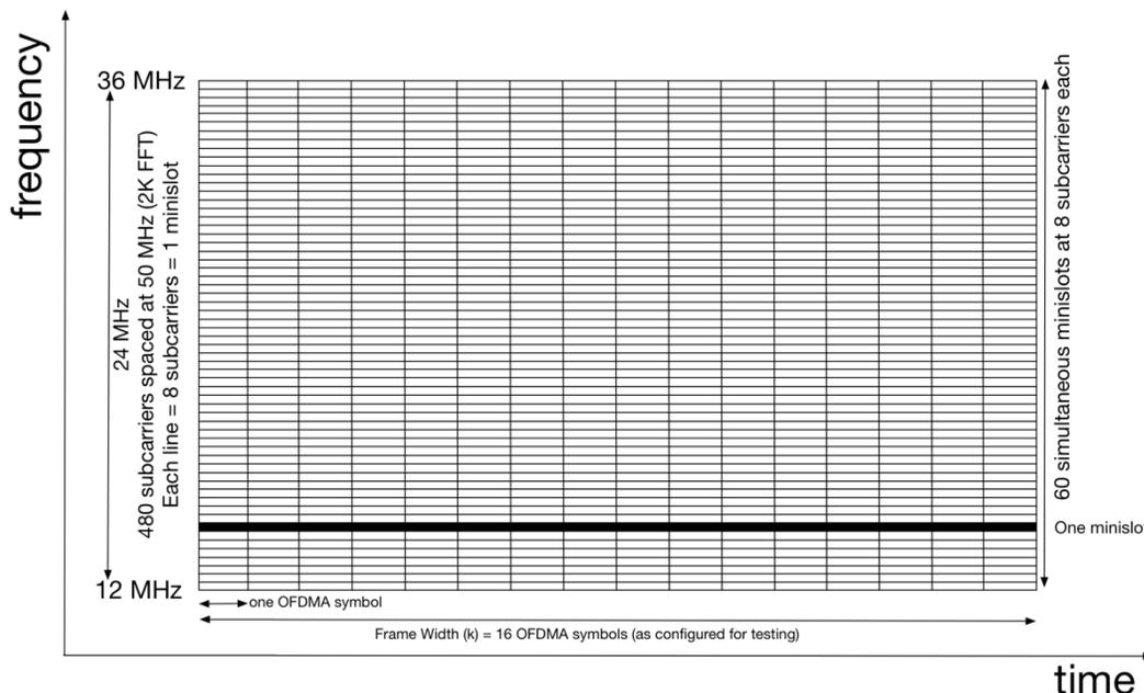
**Figure 10 – DOCSIS 3.1 Upstream OFDMA Frame Structure**
