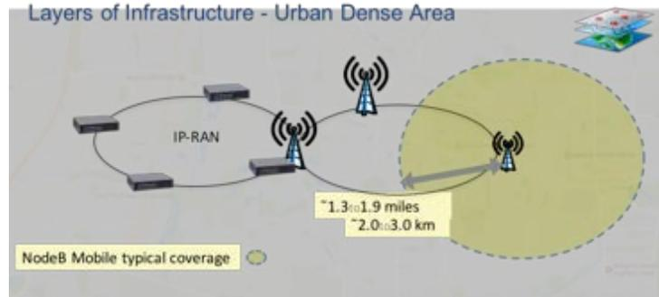
**Figure 10 – Example of an Existing Mobile infrastructure**
