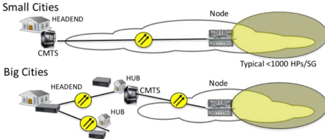
**Figure 3 – Typical Cable Access Infrastructure Implementation**
