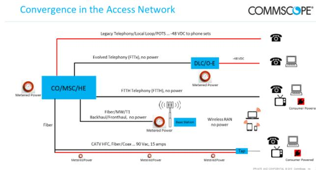
**Figure 4 - Convergence in the Access Network**
