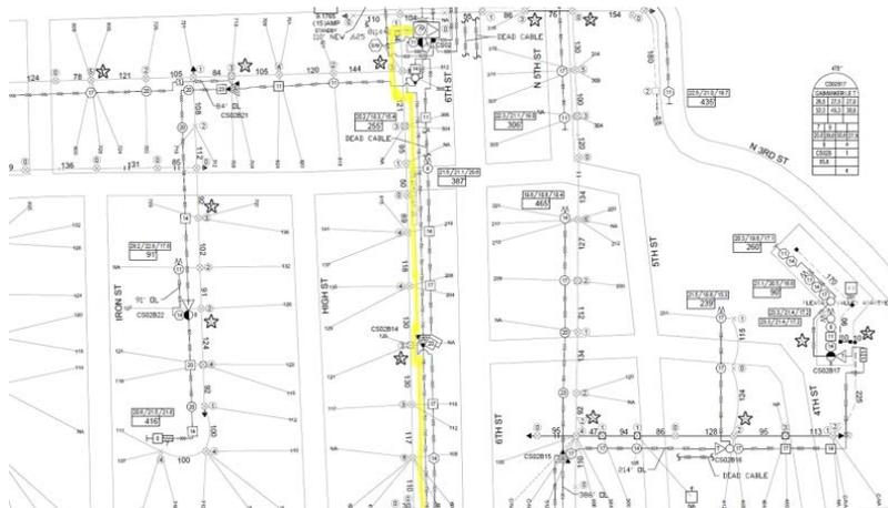
**Figure 6 - Fiber and Coaxial overlay in HFC**
