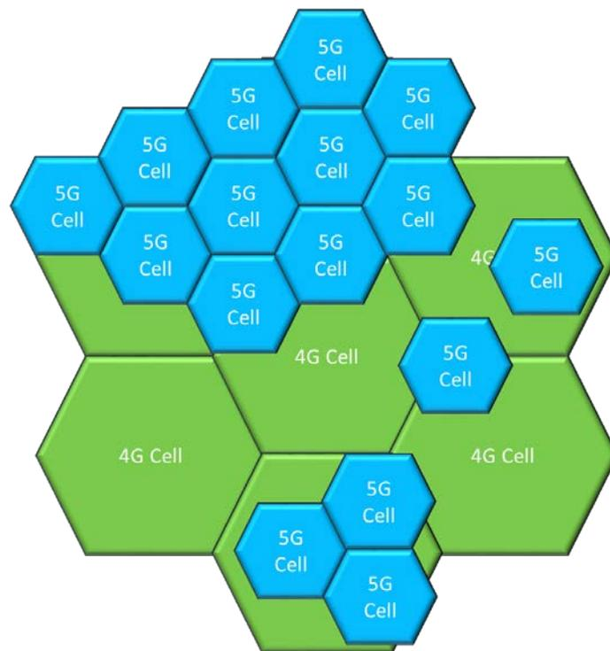
**Figure 1 - 4G and 5G Cell Coexistence. Source: Infinera**
