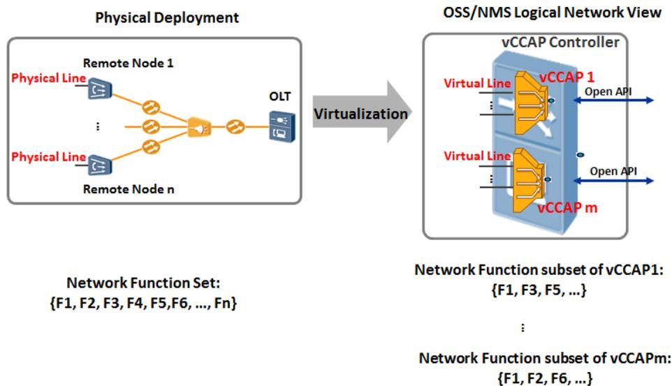
**Figure 5 - Access Network Function Virtualization and Allocation**
