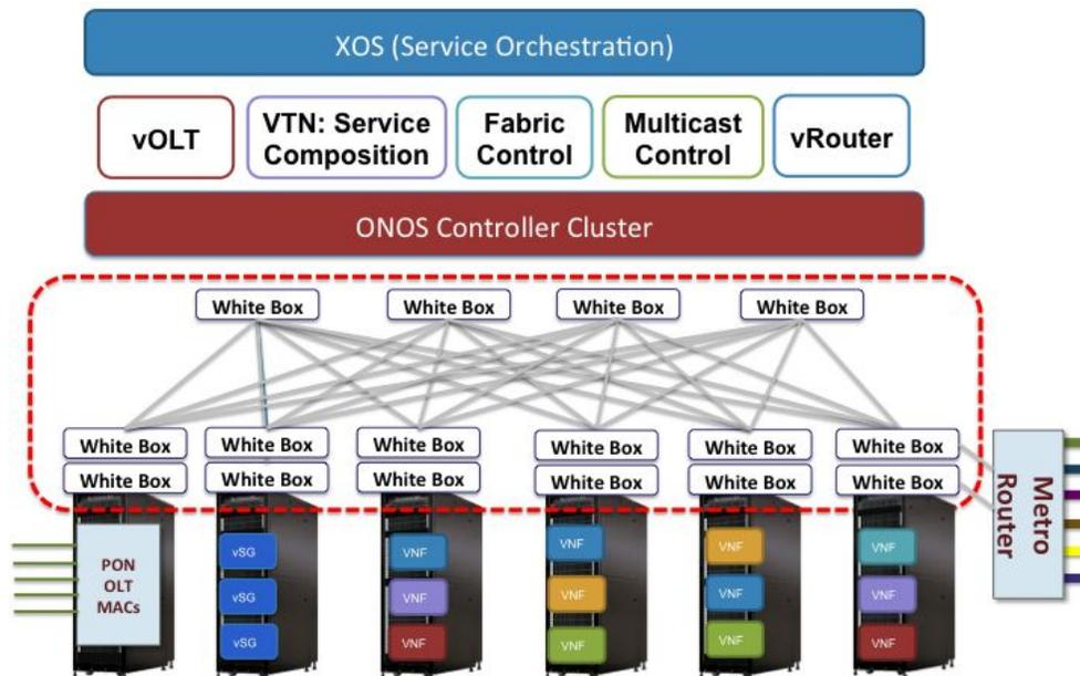
**Figure 8 - R-CORD Architecture (Das, et al., 2016)**
