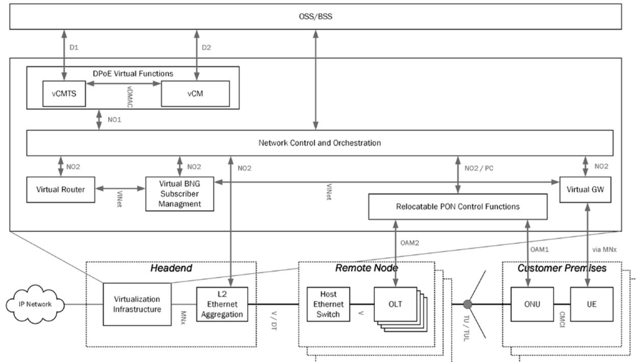
**Figure 12 - Long Range Distributed EPON Architecture**
