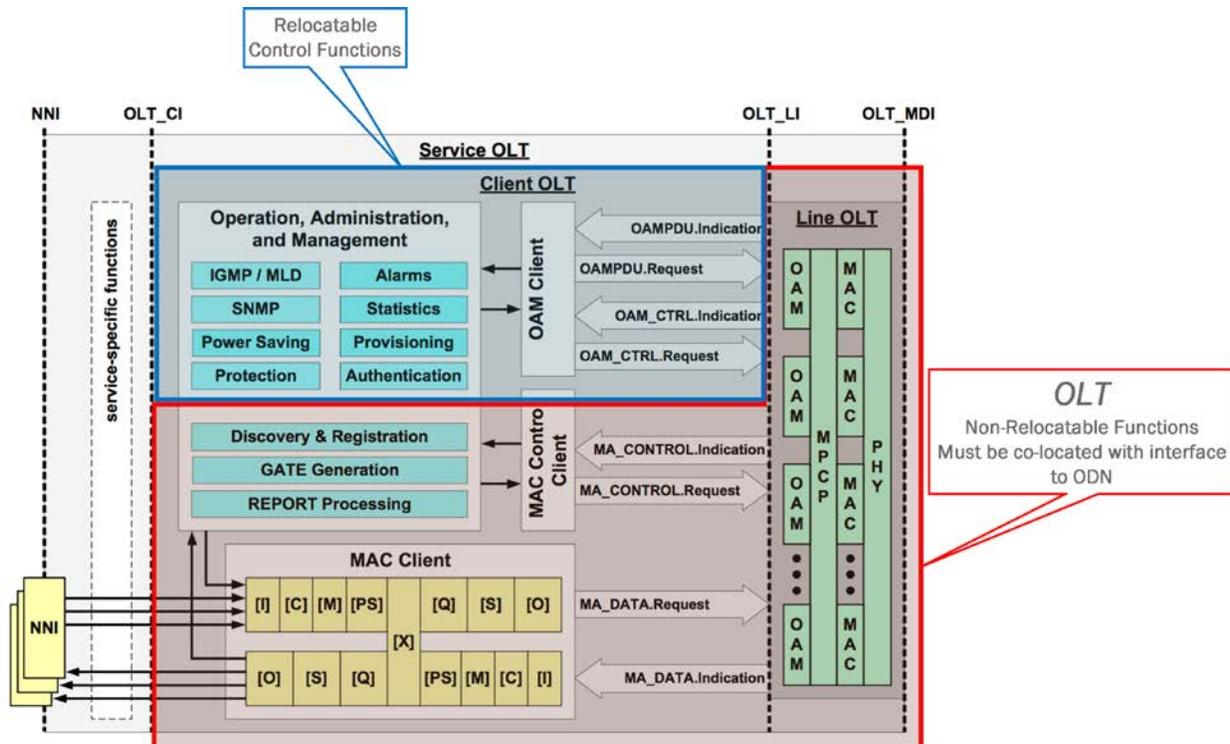
**Figure 10 - Disaggregated SIEPON S-OLT**
