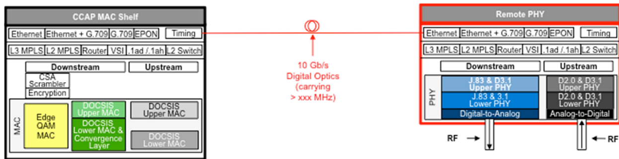
Figure 9: Remote PHY Architecture (RPA) Detailed View
