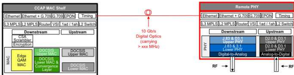
Figure 26: Remote PHY Architecture (RPA)
