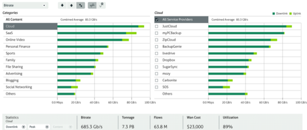
Figure 2: example visualization of services usage, classified by content category. This gives visibility towards any caching VNFs implemented on a per-content basis, and parameters such as by utilization or WAN cost allow for operational oversight. Furthermore the sites/site-pairs could be exposed to view top demand generators for each service.
