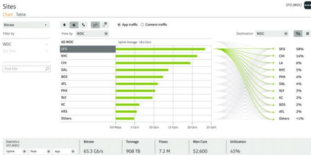
Figure 6: example visualization of site-based traffic. Site-to-site interactions give visibility towards how DCOI-based resource allocation VNFs are operating, such as those driving WAN-based network optimization.
