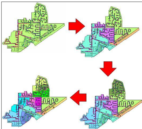
Figure 17 – Fiber Deep Segments a Serving Area
