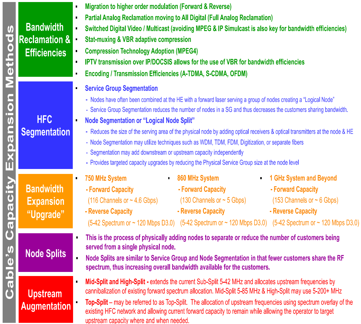
Figure 51 – Cable's Capacity Expansion Methods
