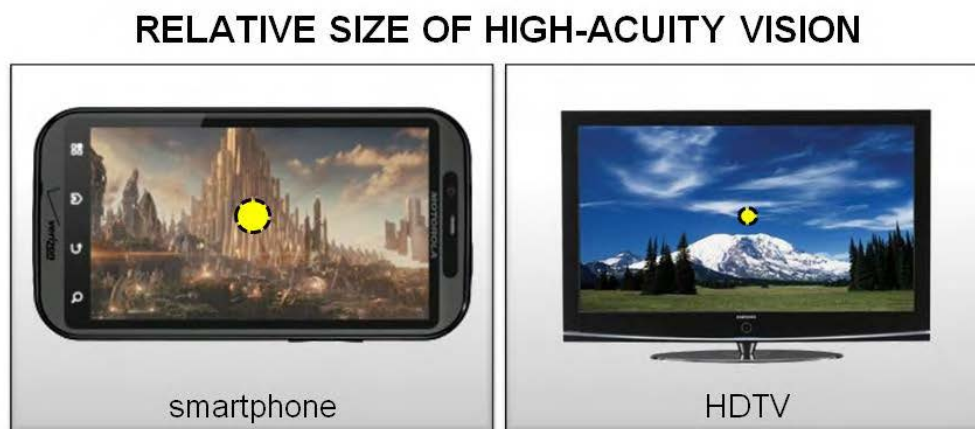
Figure 16 – Size of Projected Foveal Image (yellow) vs. Display Type
