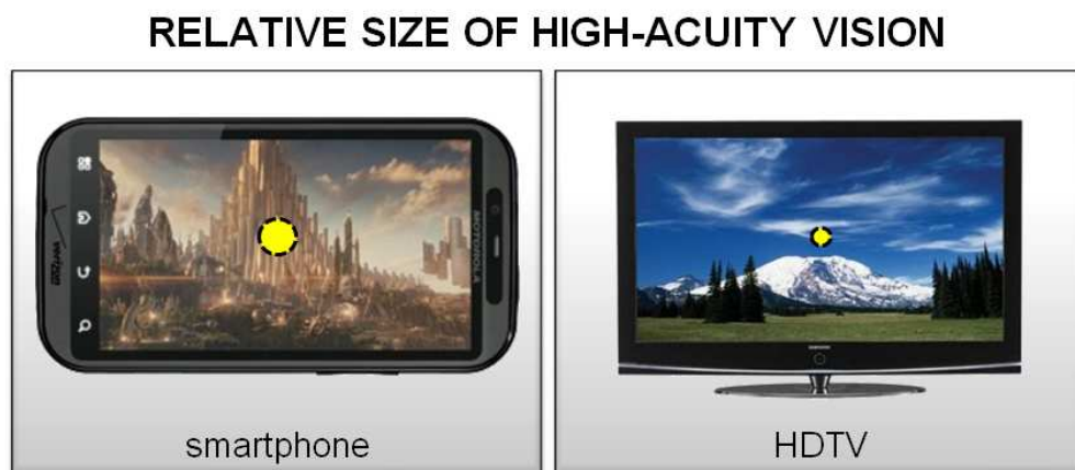
Figure 16 – Size of Projected Foveal Image (yellow) vs. Display Type
