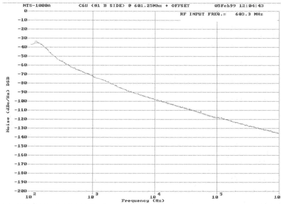
Figure 24 – Example Phase Noise Mask – RF Upconverter @ 601.25 MHz
