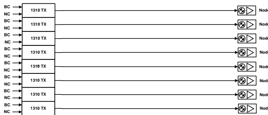
Figure 1 – Typical 1310 Hub to Node Downstream Optics
