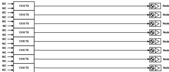
Figure 1 – Typical 1310 Hub to Node Downstream Optics
