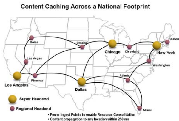
Figure 15 – Advanced content caching protocols enable real-time ingest and real-time distribution of video content across a national footprint.
