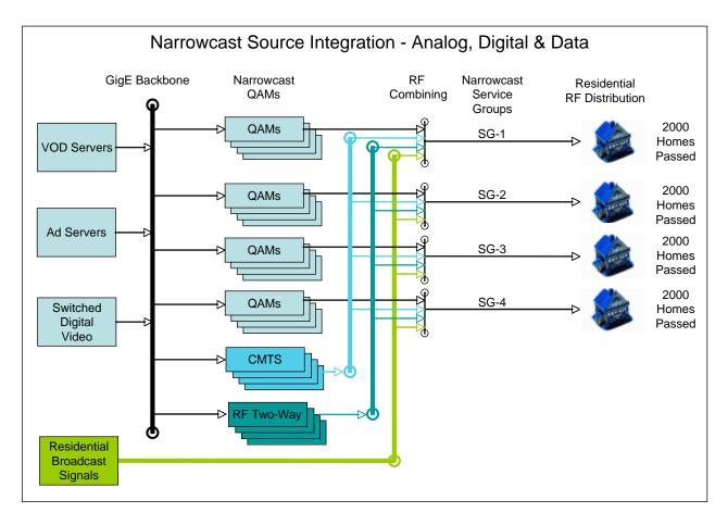
**Narrowcasting** is the narrow "broadcasting" of source signals (analog video, digital video or data) to a subset of the cable plant and not indiscriminately to the plant on the whole.
