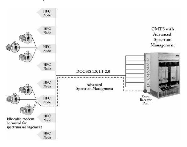
MSOs can use the extra receiver to identify the diverse types of noise and then implement spectrum management enhancements that process can this information and take measures to cancel it out in real time. The extra receiver can be effectively connected in parallel with a live receiver port so the operator can measure traffic and performance in real-time on any given live receiver port.
