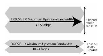
DOCSIS 2.0 doubles the channel width and triples the upstream capacity when compared with DOCSIS 1.X cable modems.
