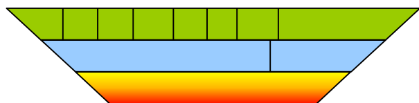
Figure 2: Layering of transport and overlay layer-2 networks on wavelength-division multiplexed (WDM) transmission.
