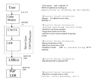
The CMTS portion of an integrated CMTS/edge router at the headend reserves the resources and schedules the traffic flows in the DOCSIS network The LSR portion of the system inspects each flow in real time, maps the packets to an MPLS LSP, applies the appropriate MPLS label and routes the traffic to an MPLS Label Switched Router (LSR) in the core network. The LSRs then switch the packets across the MPLS network to the corresponding LERs at the points of presence for the content sources.
