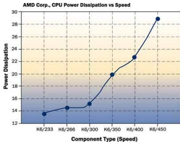
Figure 2 – AMD CPU Heat Dissipation vs. Clock Speed
