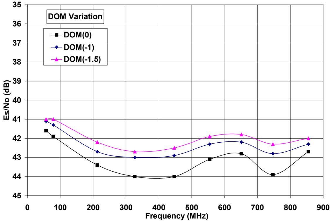
Figure 5 – 64 QAM Es/No versus Frequency for DOM Variations
