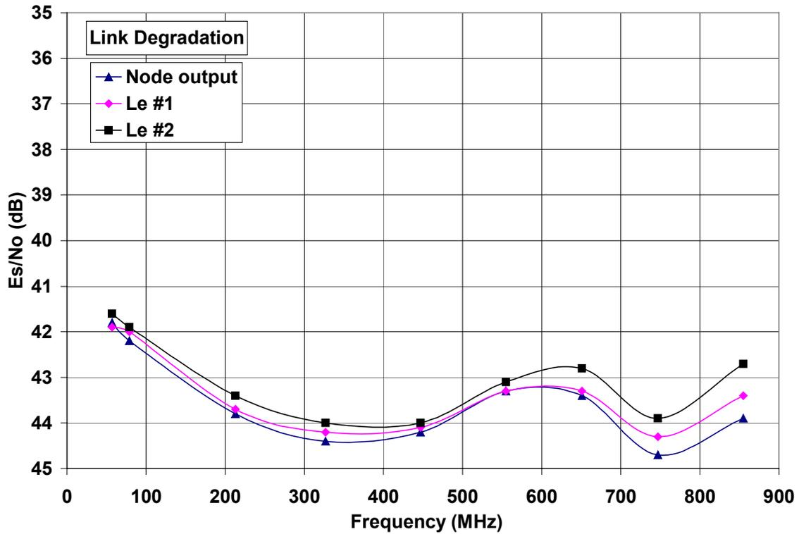
Figure 4 – Es/No versus Frequency for Distribution Depth
