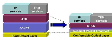
The RPT packet includes a 6 bytes RPT header and 4 bytes MPLS and contains all the necessary information to move the packet through the network. This is a very small tax relative to SONET and ATM for similar functionality.
