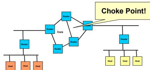
RPT eliminates the layer three bottleneck and expense by operating in Layer 2-1/2 and using the RPT header for pack destination information. As each packet traverses network, the RPT header determines if the packet should be dropped or passed. RPT enabled boxes will likely reduce network dependence on high capacity routers.
