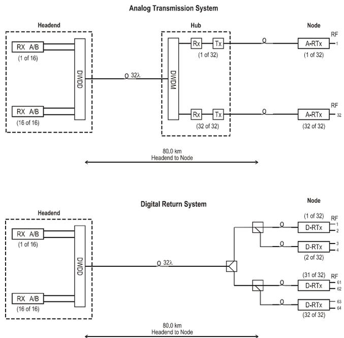
Figure 1. Comparison of analog and digital return transmission system architectures
