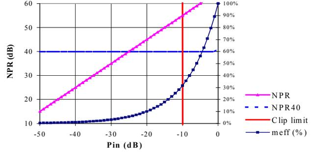
Figure 2. NPR and  $\mu_{\text{eff}}$  as a function of RF power
